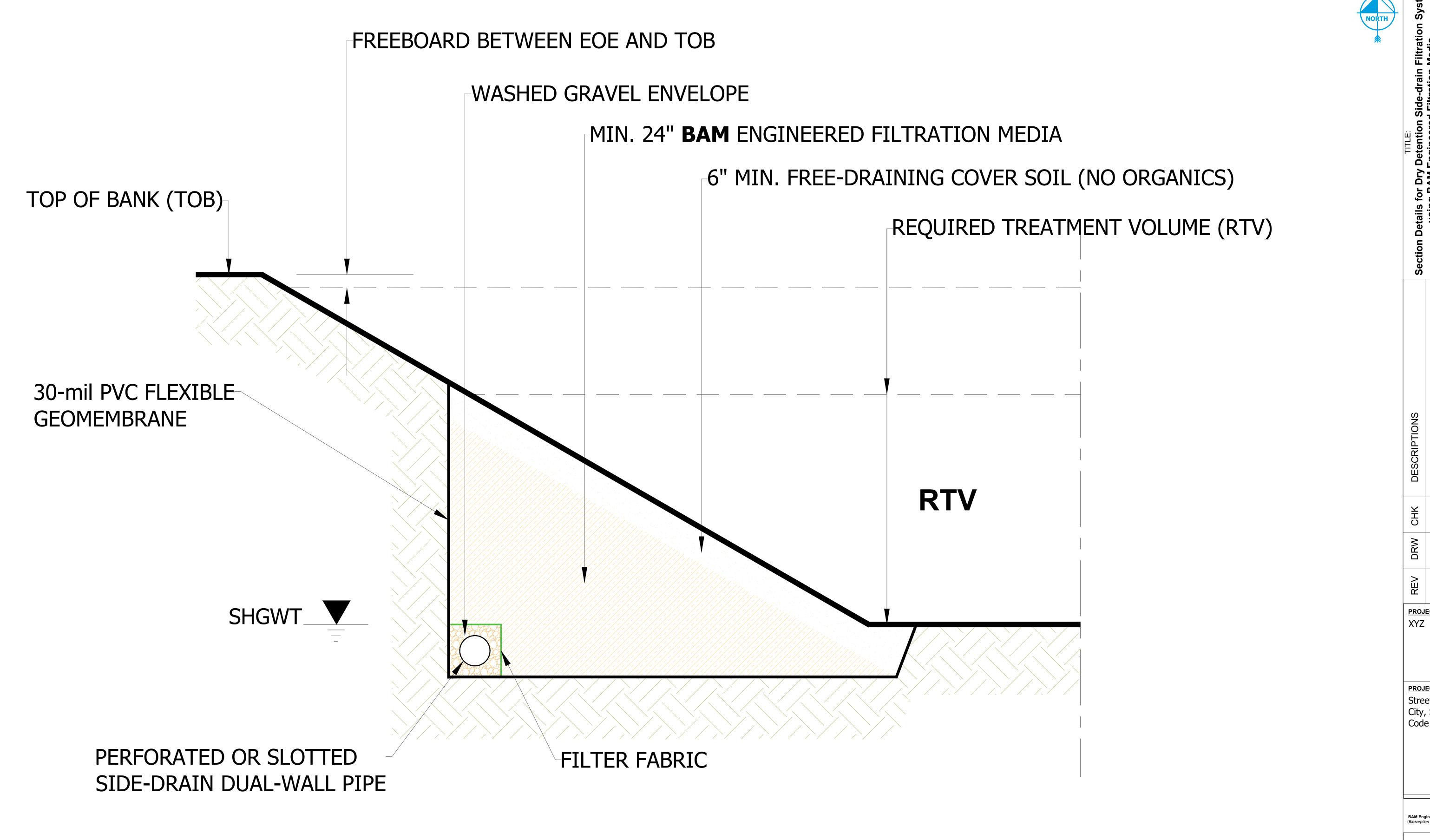
BAM ENGINEERED FILTRATION MEDIA USED AS A FILTER MEDIA AT THE BANK OF A POND
